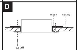
Use a hand to hold the mesh down whilst fixing the collar in place with drywall screws. All eight screws must be used to avoid risk of the plaster cracking.
