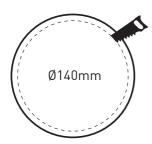
Cut a Ø140mm circular hole at the desired location using a holesaw.
