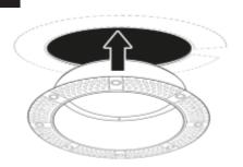
Fit the plaster-in collar into the hole.
